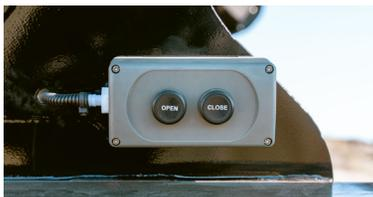
Walk along gate control located on the hopper sidewall
